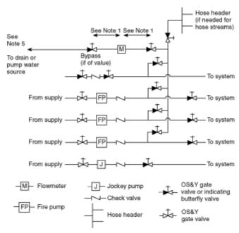
Figure A-2-14.1.2(b) Typical arrangement for measuring fire pump water flow with meter. Discharge from the flowmeter is recirculated to the fire pump suction line.
