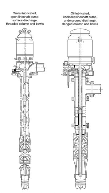
Figure A-4-2.2.1 Vertical shaft turbine-type pump installation in a well.
