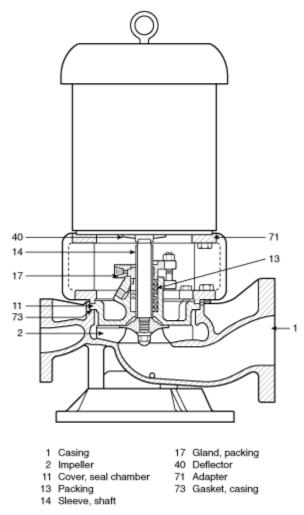
Figure A-3-1.1(d) Overhung impeller — separately coupled single stage — in-line — rigid coupling.
