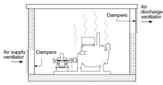
Figure A-8-3.2(b) Typical ventilation system for a radiator-cooled diesel-driven pump.
