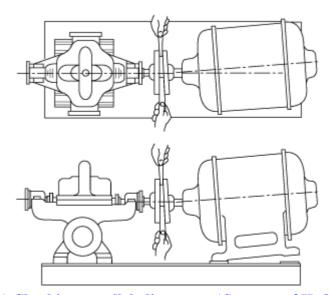
Figure A-3-5(b) Checking parallel alignment. (Courtesy of Hydraulics Institute
