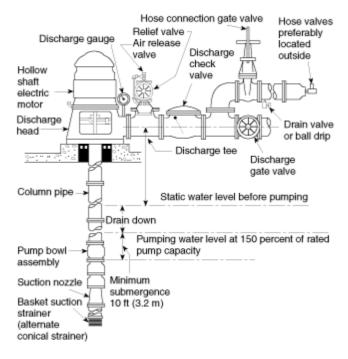
Note: The distance between the bottom of the strainer and the bottom of the wet pit should be one-half of the pump bowl diameter but not less than 12 in. (305 mm).
