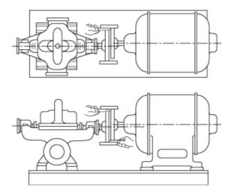
The unit should be checked periodically for alignment. If the unit does not stay in line after being properly installed, the following are possible causes:
