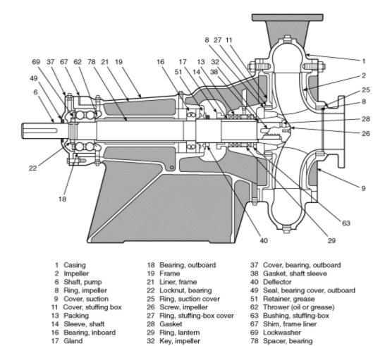
Figure A-3-1.1(c) Overhung impeller — close coupled single stage — in-line (showing seal and packaging).
