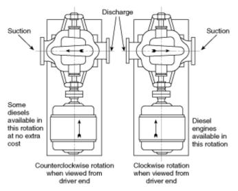
(c) Vertical Pump Shaft Rotation. The rotation of a vertical pump can be determined by looking down upon the top of the pump. [See Figure A-2-17(c).] If the point of the shaft directly opposite revolves from left to right, the rotation is right-handed [or clockwise (CW)]. If the point of the shaft directly opposite revolves from right to left, the rotation is left-handed [or counterclockwise (CCW)].
