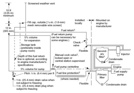
Secondary filter behind or before engine fuel pump, according to engine manufacturer's specifications.
