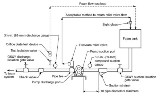
Figure A-5-4.4 Typical water mist system pump piping and fittings.
