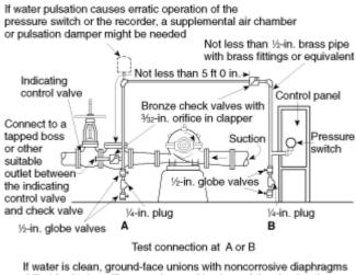
drilled for 3/22-in. orifices can be used in place of the check valves.
