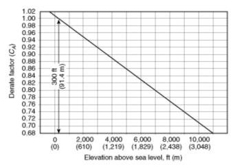
Note: Correction equation: Corrected engine horsepower =  $(C_A + C_T - 1) \times \text{Listed}$  engine horsepower
