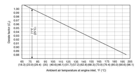
Note: Correction equation: Corrected engine horsepower =  $(C_A + C_T - 1) \times$  Listed engine horsepower
